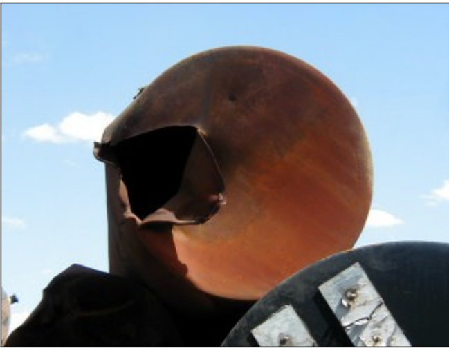
Acceptable: Large openings on tanks for inspection
