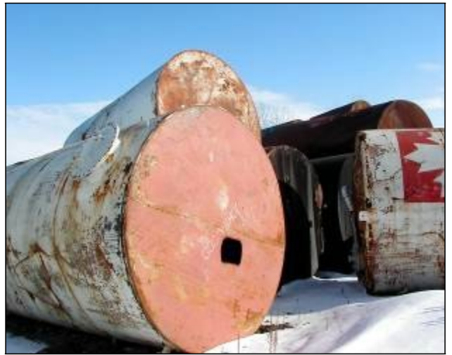
Acceptable: Large openings on tanks for inspection
