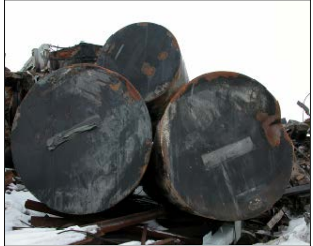
Prohibited: No openings on the tanks for inspection
