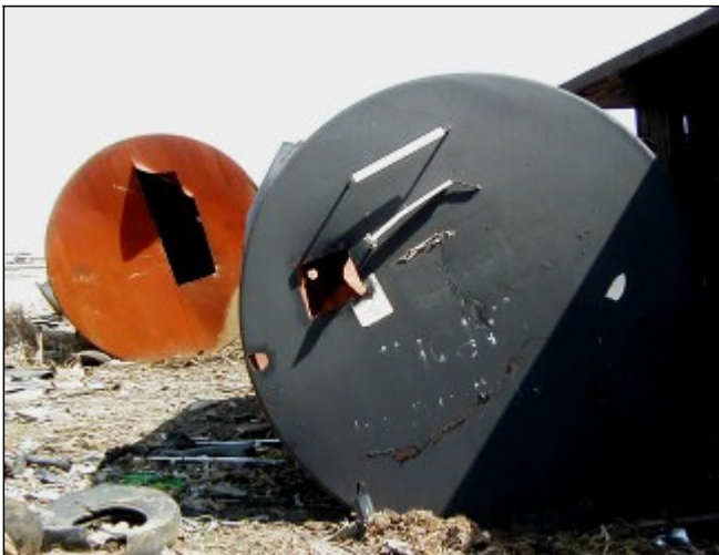
Acceptable: Large openings on tanks for inspection
