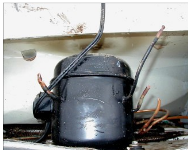
Acceptable: CFC/Freon drained and lines cut prior to delivery
