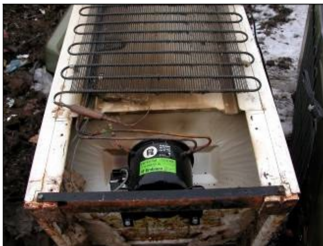
Prohibited: If Freon/CFC system is intact
