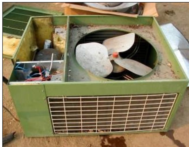
Prohibited: If Freon/CFC system is intact
