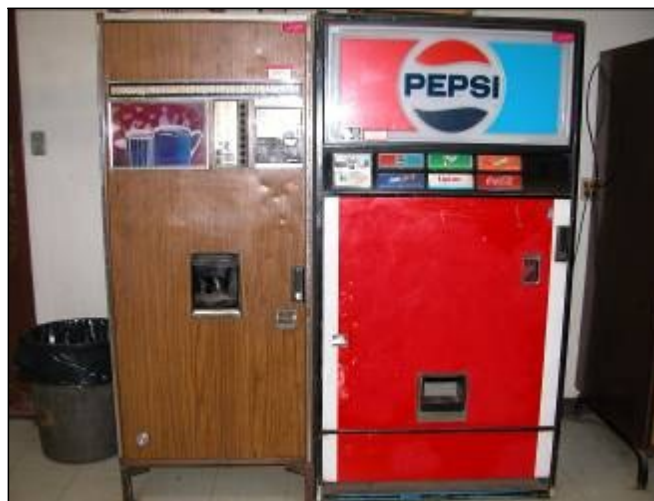
Prohibited: If Freon/CFC system is intact
