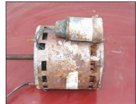
Prohibited: Capacitor in AC motors
