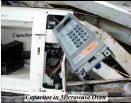
Prohibited: Capacitor in microwave oven
