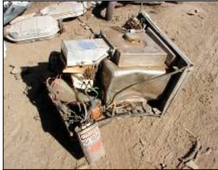
Prohibited: Capacitor in microwave oven
