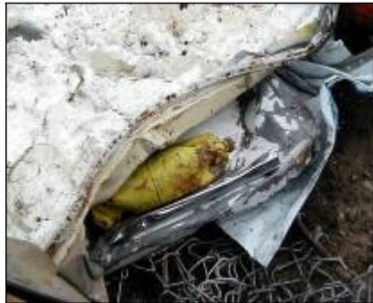
Prohibited: Propane bottle inside a vehicle
