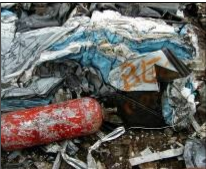
Prohibited: Propane bottle inside a bale
