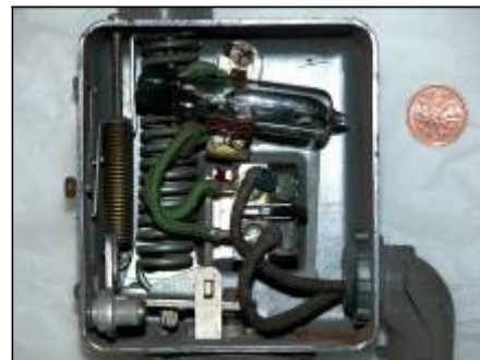
Prohibited: Mercury in pressure and temperature gauges
