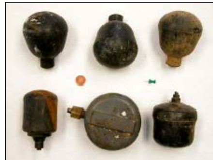
Prohibited: Mercury in level switches
