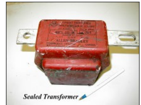
Prohibited: Sealed transformer
