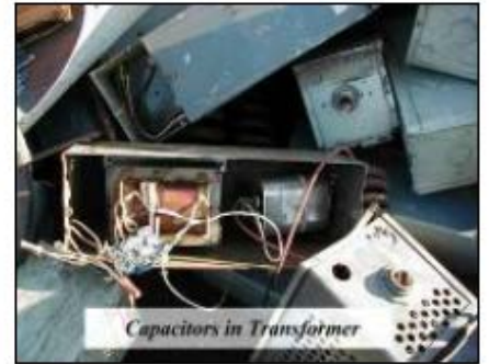
Prohibited: Capacitors in transformer
