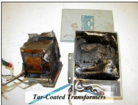
Prohibited: Tar-coated transformer
