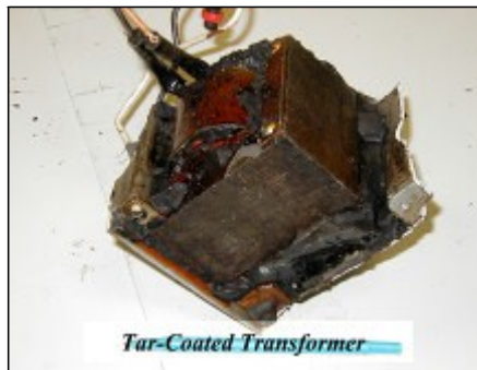
Prohibited: Tar-coated transformer
