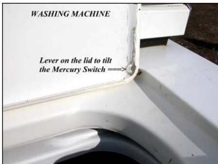
Washing machine with mercury switch
