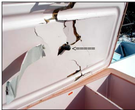
Mercury switch in a freezer
