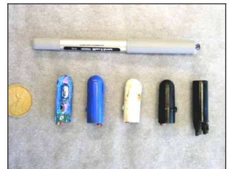
Mercury switches from washing machines
