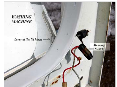
Mercury switch in a washing machine
