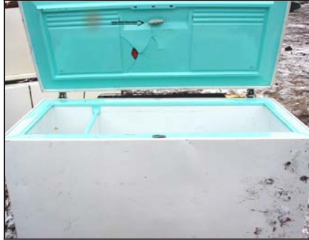
Mercury switch in a freezer
