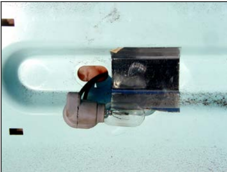
Mercury switch in a freezer
