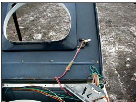
Mercury switch in a washing machine
