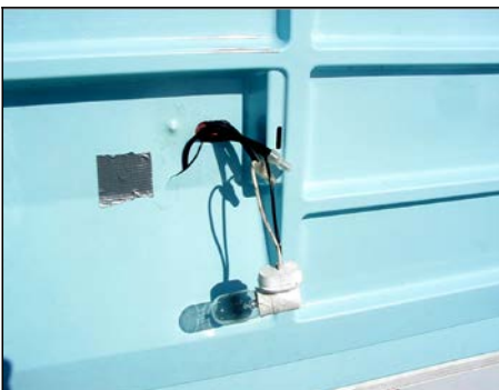
Removing mercury switch in a freezer
