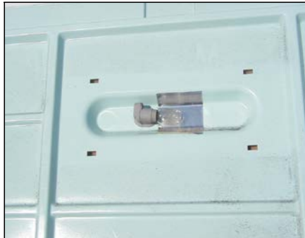
Mercury switch in a freezer
