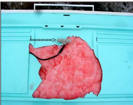
Mercury switch in a freezer
