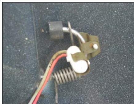
Mercury switch in a washing machine
