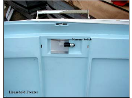
Mercury switch in a freezer
