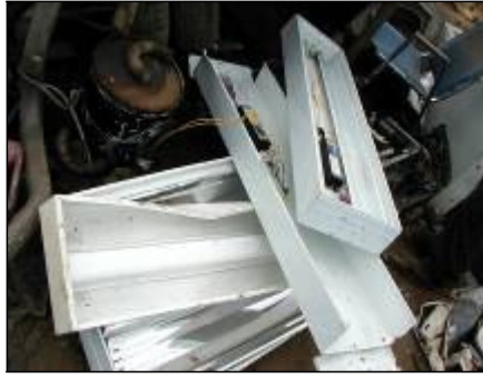
Prohibited: Ballasts on fluorescent light fixtures
