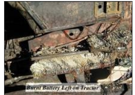
Prohibited: Battery left in a burnt tractor
