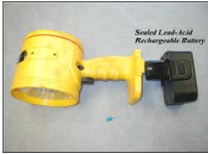
Prohibited: Rechargeable sealed lead-acid battery co-mingled with other scrap
