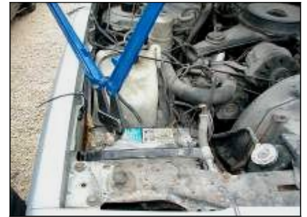
Prohibited: Lead-acid battery left in a vehicle
