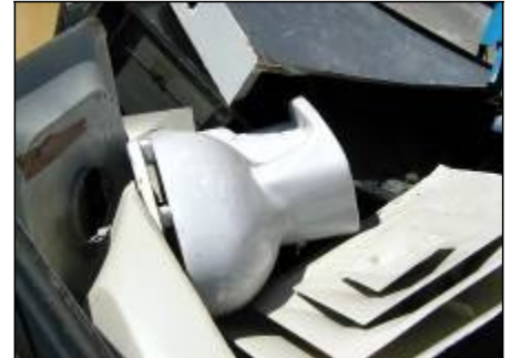
Prohibited: Non-metallic materials inside crushed vehicle
