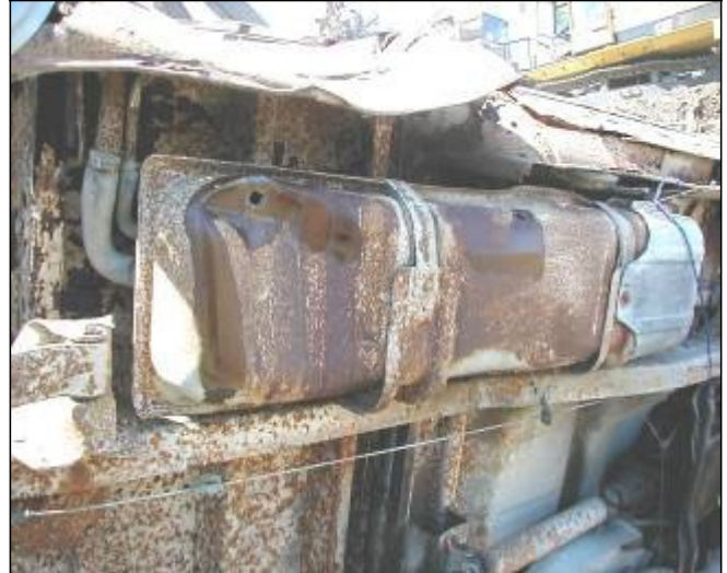
Acceptable: Gas tank on vehicle drained and punctured with two large holes at lowest points prior to delivery to the facility
