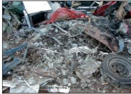
Prohibited: Non-metallic materials inside crushed vehicle
