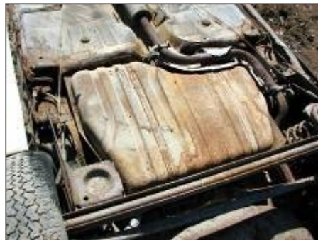
Prohibited: Un-punctured gas tank on vehicle
