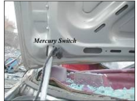
Prohibited: Mercury switch in trunk
