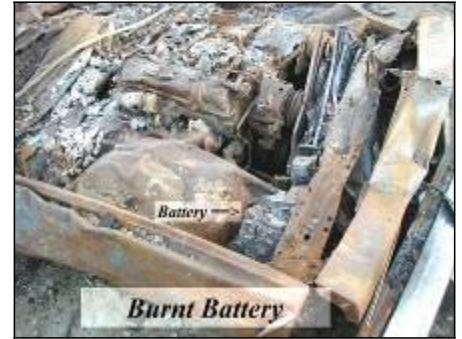
Prohibited: Lead-acid battery left in a vehicle
