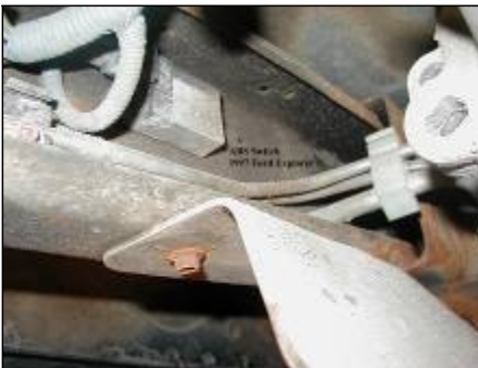
Prohibited: ABS mercury-containing switch located on the chassis on the underside of vehicle
