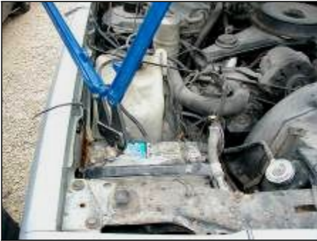
Prohibited: Lead-acid battery left in a vehicle
