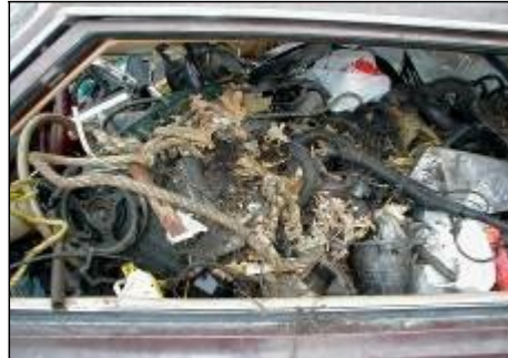
Prohibited: Non-metallic materials inside vehicle
