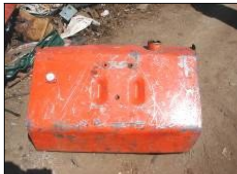
Prohibited: Un-punctured miscellaneous fuel tank
