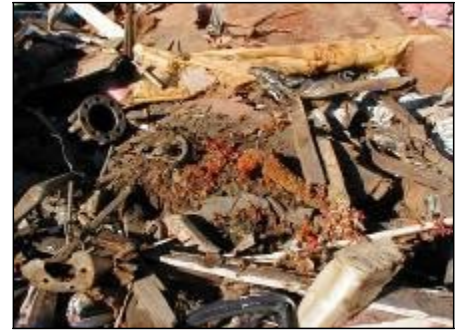
Prohibited: Non-metallic materials inside crushed vehicle
