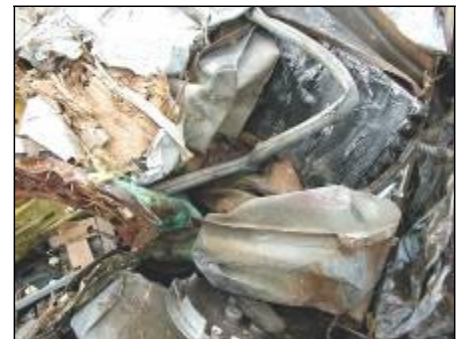
Prohibited: Un-punctured gas tank commingled with other scrap
