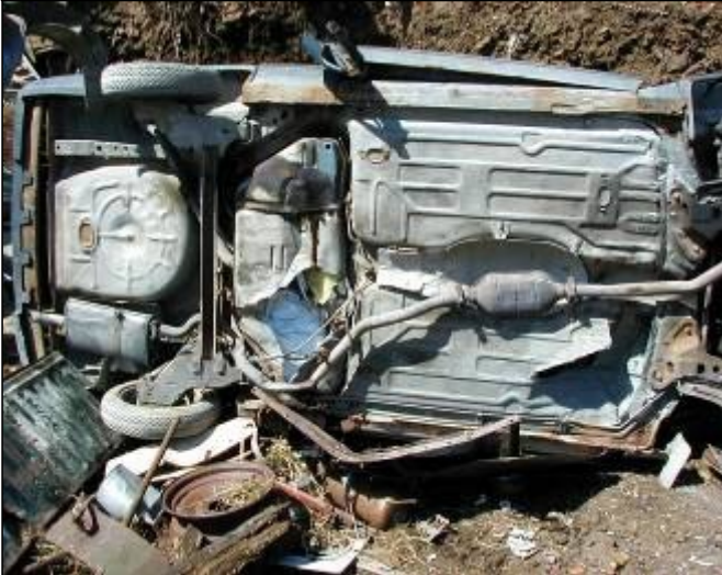
Acceptable: Gas tank on vehicle slit wide open prior to delivery to the facility
