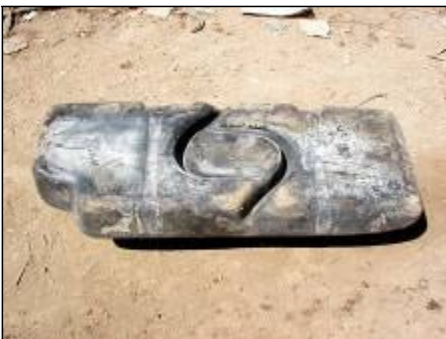
Prohibited: Un-punctured gas tank
