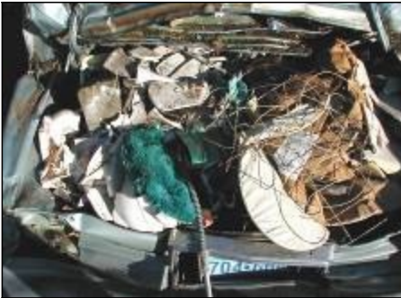
Prohibited: Non-metallic materials inside trunk of crushed vehicle
