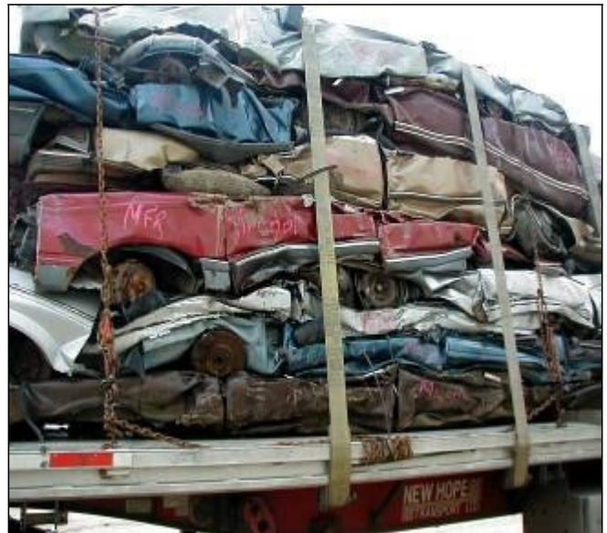
Acceptable: Every vehicle must be marked with customer specific identification number and the letters "mfr" or "mf"
